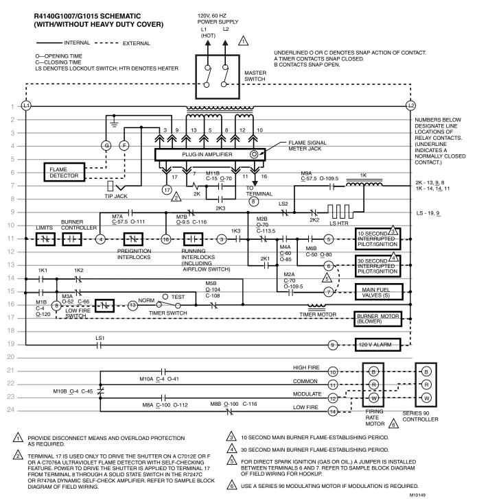
Fig. 3. Simplified schematic diagram of R4140G1015 Programmer.
